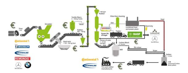
This diagram presents an example of how one tonne of end-of-life tyres is processed. In order to guarantee the product safety and quality of its end products, Pyrum operates its own tyre shredder. The volume flow and the quality of the input materials can thus be managed and monitored in a targeted manner.
