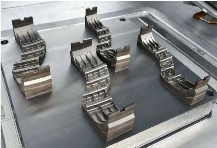
Temporary molds used to research metal 3D printing
